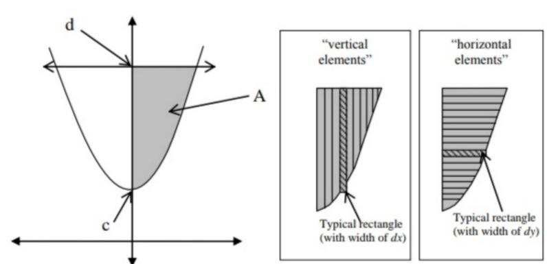
There are two ways to solve this problem: we can calculate the area between two functions y = 4 and  $y = x^2 + 2$  using the vertical elements and integrate with respect to x, or we can use the horizontal elements and calculate the area between the y-axis and the function  $y = x^2 + 2$  integrating the functions with respect to y.
