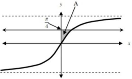
Since it is much easier to integrate  $x = \tan y$  than  $y = \arctan x$ , we will rewrite the given function in terms of y, and integrate using the horizontal elements and the formula:
