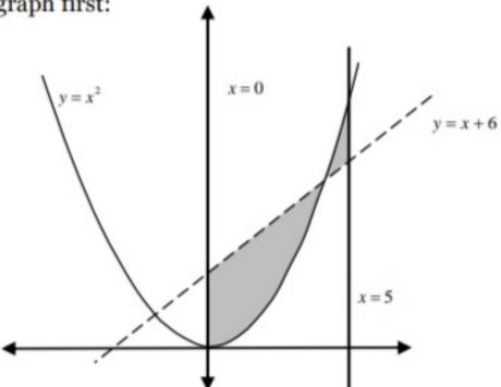
In this case it is very important to draw the graph, since the functions intersect between the boundaries. This means that we will have to actually calculate two separate integrals and then add the results. Otherwise we would end up subtracting the two pieces from each other.
